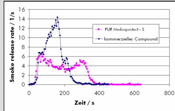
While normal sheath materials quickly release high levels of energy and smoke in the event of a fire (values shown in blue in the graph), PUR-Medoxprotect-S from Nexans burns slowly. As a result, considerably less heat and smoke develops in the first few minutes. The new sheath material is to be used for the first time in sensor cabling.
