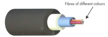
Most of the time, a tube contains a maximum of 12 fibres. In case of higher fibre count, an additional ring marking is added on the fibre coating.
