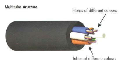
When there are several tubes in the cable, the EIA colour standard can also apply to the different tubes. Alternatively, there is as well the possibility to have the same colour for all the tubes, but with a different marking on each one.
